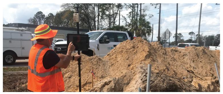
A NSBU mobile worker collects assets using ArcGIS® apps on iPad® with an Eos Arrow Gold® GNSS receiver on a rangepole.
