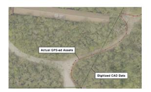
NSBU quickly realized that their CAD as-built records did not match the real assets. The digitized CAD data (green line) was extremely inaccurate when compared to the actual GPS'ed assets (red line).
