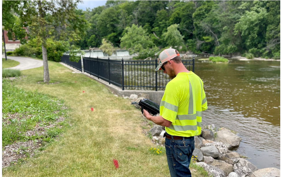
SFU line worker Justin Kiecker maps primary underground linear assets with submeter accuracy. Points (marked in red spray paint) were later digitized into lines, using the ArcGIS snap feature.
